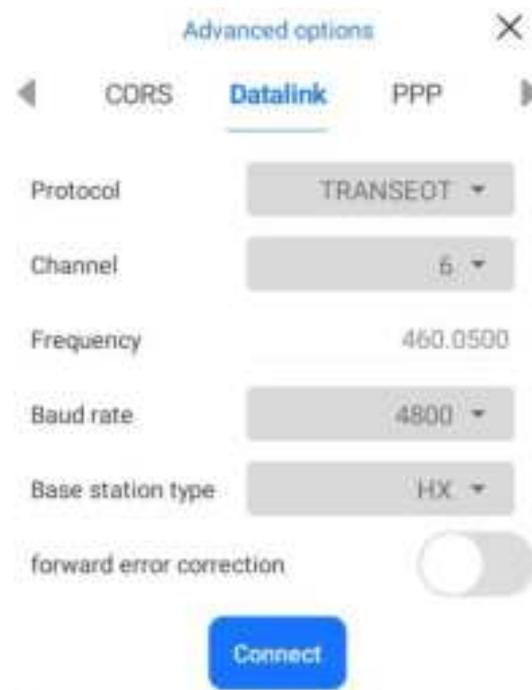
And if you want to use another protocol or other brand's receiver as mobile base station, Please make sure that the protocol, frequency, and baud rate settings of the tablet and mobile base station are exactly the same.
