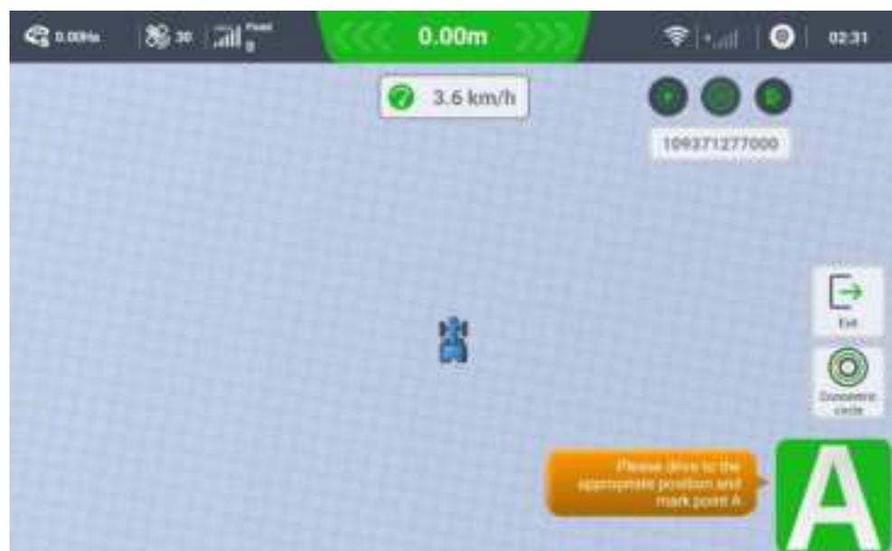
Input the minimum radius between adjacent circles, or drive the car to the target position and get the distance
