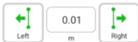
Supports moving the guide line to the left or right of the direction of the front of the vehicle according to the value manually entered by the customer (unit: meters)
