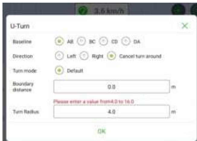
When the tractor is in the area, turn on the autosteer, and when it is about to reach the intersection of the Job line and the boundary, it will automatically turn around according to the set parameters.
