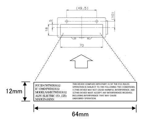
\*The way of attaching FCC ID is "Seal". Material of seal is PET.
