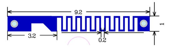
Antenna Type: PCB Antenna
