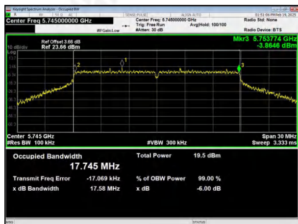
(802.11ac20) 6dB Bandwidth plot on channel 149
