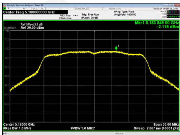
(802.11ac20) PSD plot on channel 40
