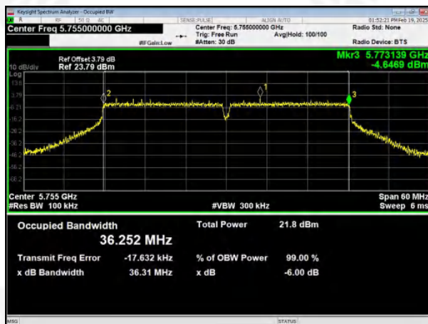
(802.11n40) 6dB Bandwidth plot on channel 151
