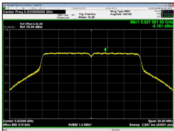
(802.11n20) PSD plot on channel 165
