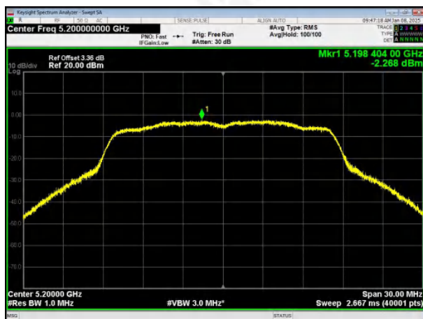
(802.11a) PSD plot on channel 40
