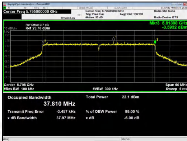
(802.11ax80) Bandwidth plot on channel 155
