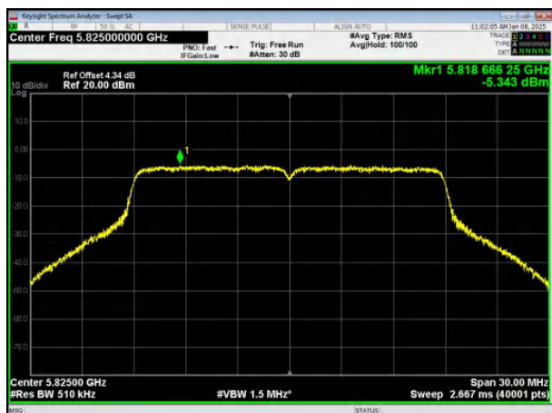
(802.11ac20) PSD plot on channel 165
