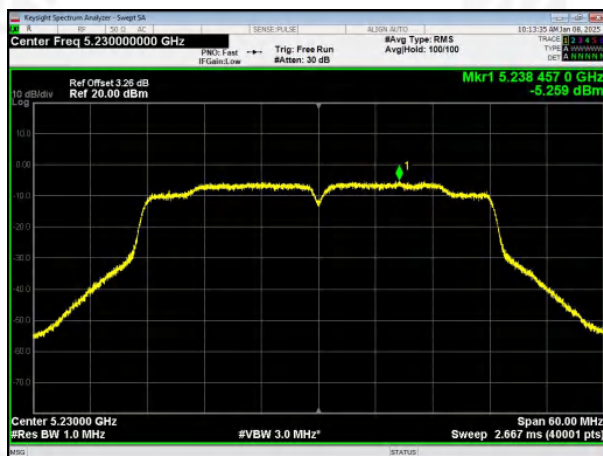
(802.11ac40) PSD plot on channel 46
