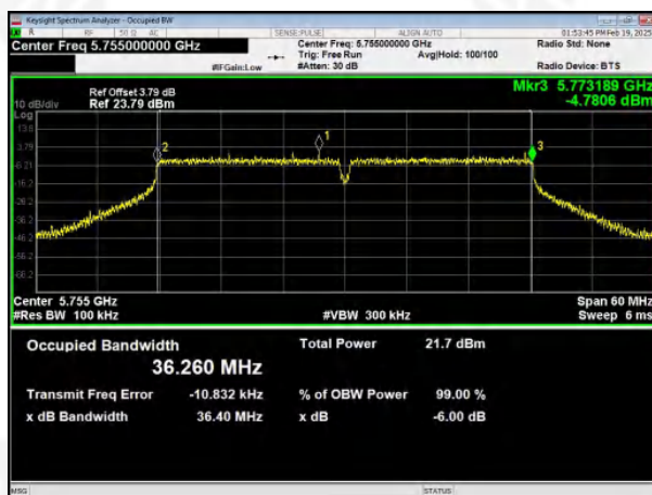
(802.11ac40) Bandwidth plot on channel 151
