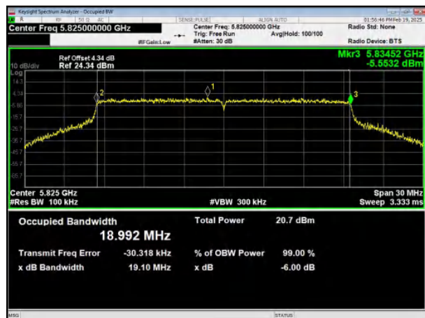
(802.11ax20) 6dB Bandwidth plot on channel 165
