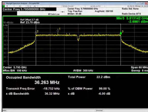
(802.11n40) 6dB Bandwidth plot on channel 159
