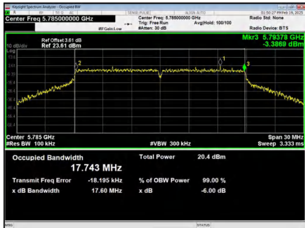
(802.11n20) 6dB Bandwidth plot on channel 165
