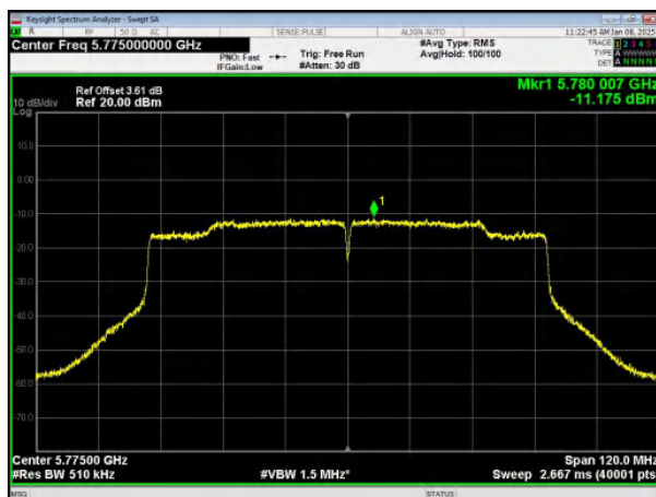
(802.11ac80) PSD plot on channel 155
