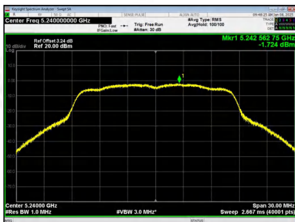
(802.11a) PSD plot on channel 48
