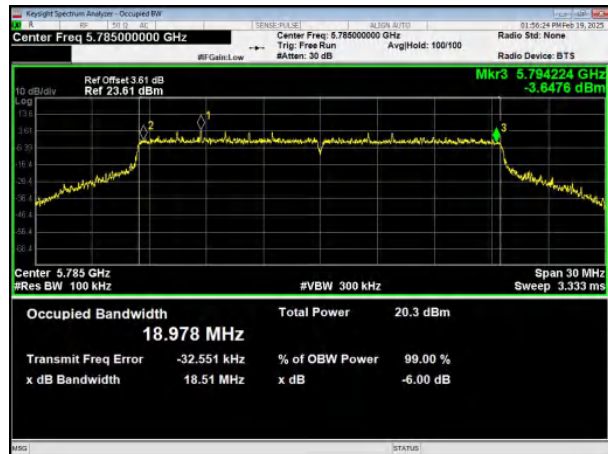
(802.11ax20) 6dB Bandwidth plot on channel 165
