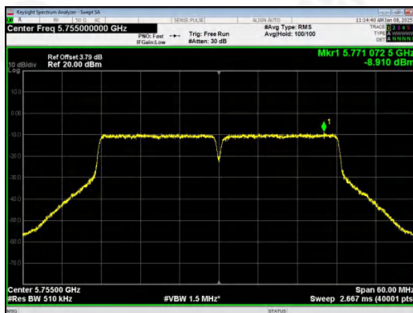
(802.11ac40) PSD plot on channel 151
