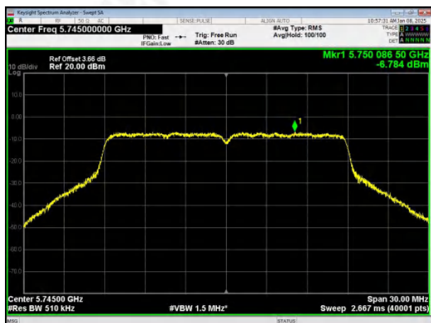
(802.11ac20) PSD plot on channel 149
