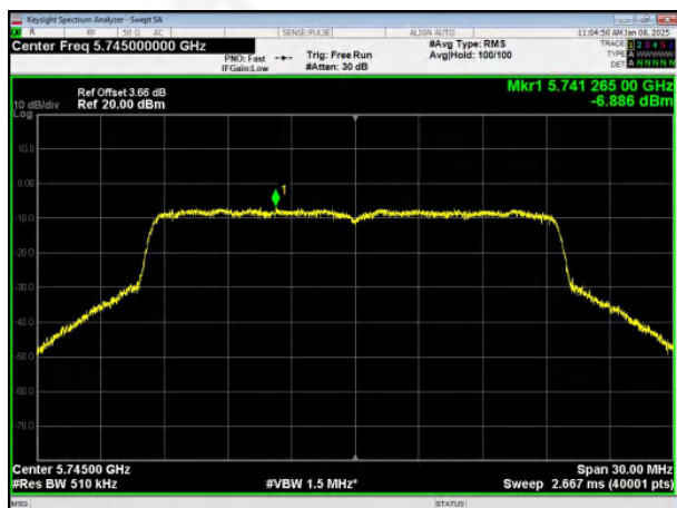
(802.11ax20) PSD plot on channel 157
