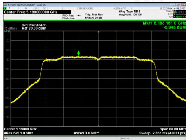
(802.11ax40) PSD plot on channel 46
