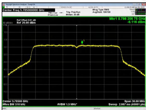
(802.11ax20) PSD plot on channel 165
