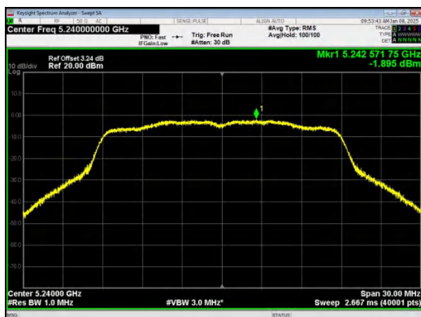
(802.11n20) PSD plot on channel 48
