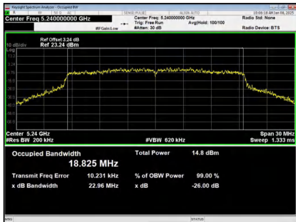
(802.11 ax20) 26dB Bandwidth plot on channel 48
