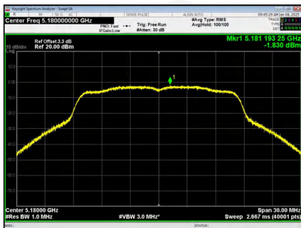
(802.11a) PSD plot on channel 36
