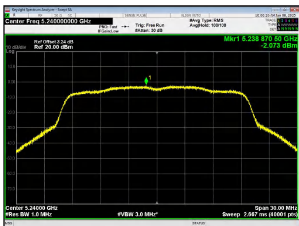
(802.11ax20) PSD plot on channel 48
