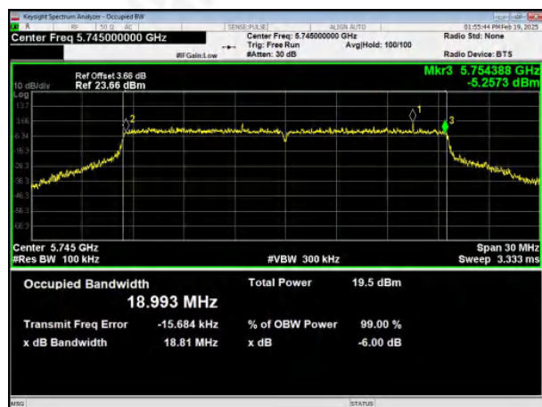
(802.11ax20) 6dB Bandwidth plot on channel 149
