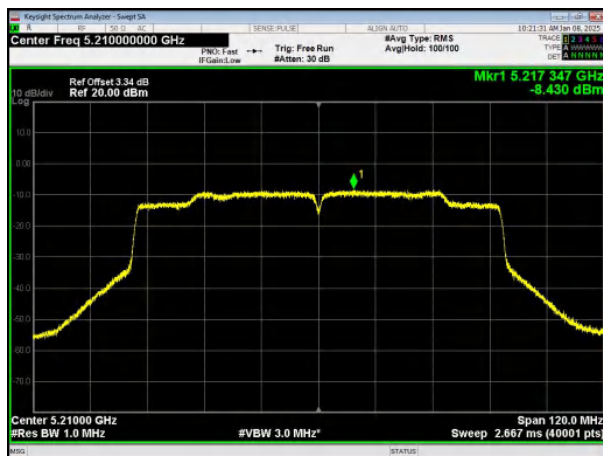
(802.11ac80) PSD plot on channel 42
