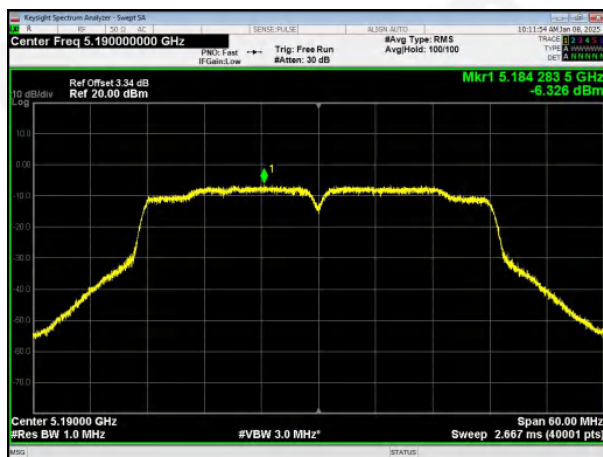
(802.11ac40) PSD plot on channel 46
