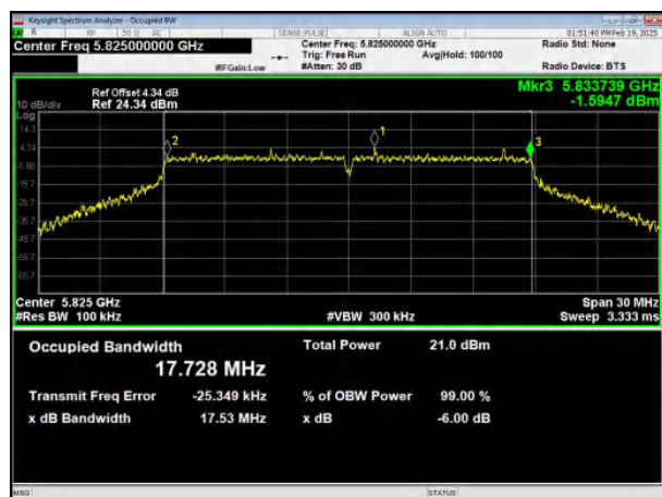
(802.11ac20) 6dB Bandwidth plot on channel 165
