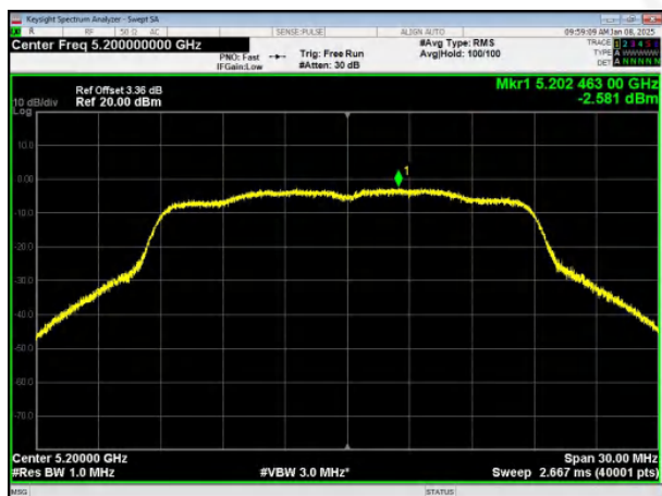
(802.11ac20) PSD plot on channel 40
