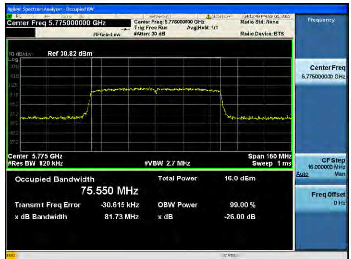
802.11ac_VHT80 UNII 3 BAND 26 dB Bandwidth (CH 155)
