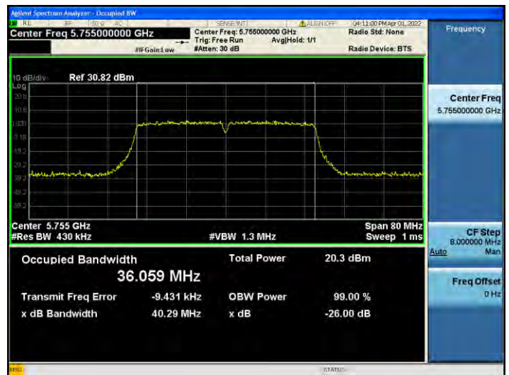
802.11ac_VHT40 UNII 3 BAND 26 dB Bandwidth (CH 151)
