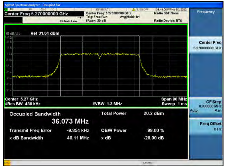
802.11ac_VHT40 UNII 3 BAND 26 dB Bandwidth (CH 159)
