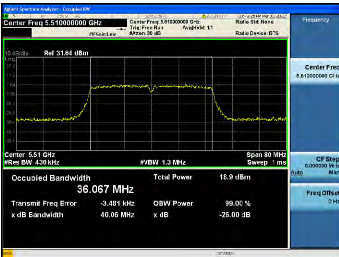
802.11ac_VHT40 UNII 2C BAND 26 dB Bandwidth(CH 102)
