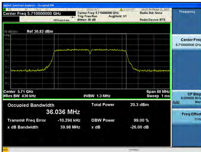
802.11n_HT40 UNII 2C BAND 26 dB Bandwidth(CH 142)
