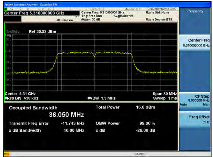
802.11ac_VHT40 UNII 3 BAND 26 dB Bandwidth (CH 151)
