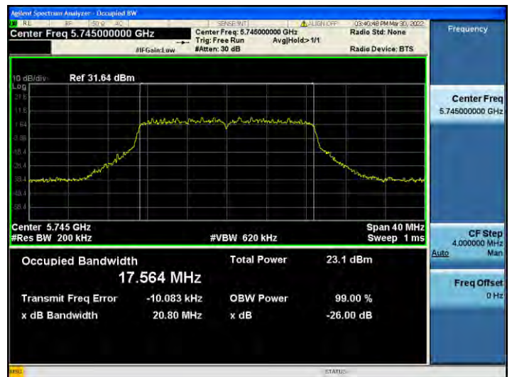
802.11n_HT20 UNII 3 BAND 26 dB Bandwidth(CH 149)
