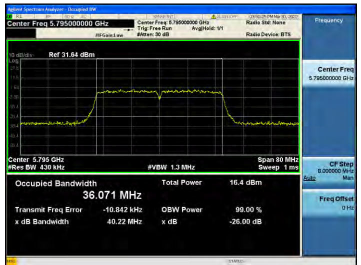
802.11ac_VHT40 UNII 3 BAND 26 dB Bandwidth (CH 159)
