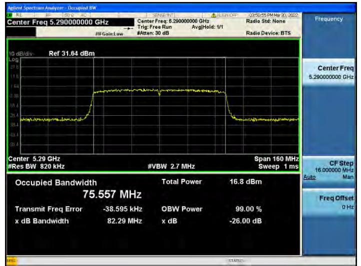
802.11ac_VHT80 UNII 3 BAND 26 dB Bandwidth (CH 155)
