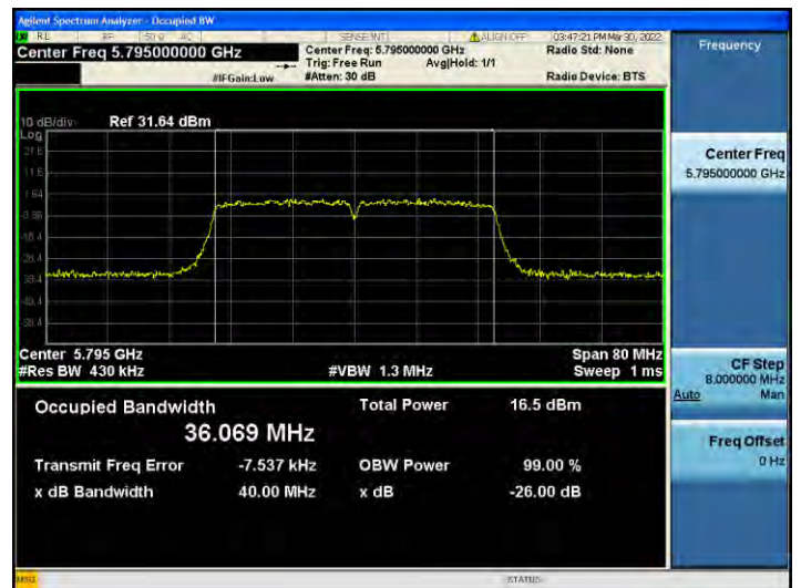
802.11n_HT40 UNII 3 BAND 26 dB Bandwidth (CH 159)
