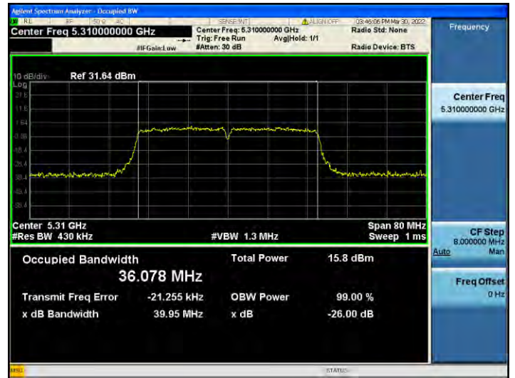
802.11n_HT40 UNII 3 BAND 26 dB Bandwidth (CH 159)
