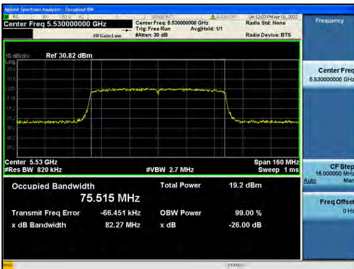
802.11ac_VHT80 UNII 2C BAND 26 dB Bandwidth(CH 106)
