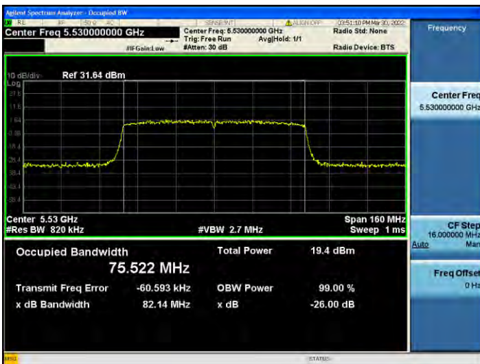
802.11ac_VHT80 UNII 2C BAND 26 dB Bandwidth(CH 106)
