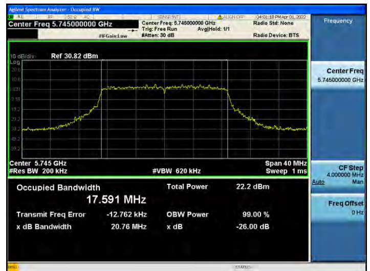
802.11n_HT20 UNII 3 BAND 26 dB Bandwidth(CH 149)
