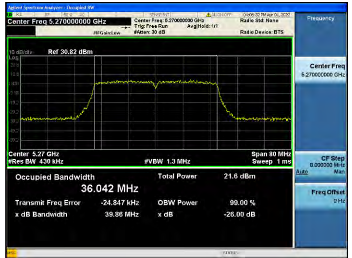
802.11n_HT40 UNII 3 BAND 26 dB Bandwidth (CH 159)
