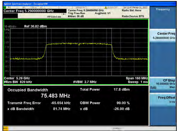
802.11ac_VHT80 UNII 3 BAND 26 dB Bandwidth (CH 155)
