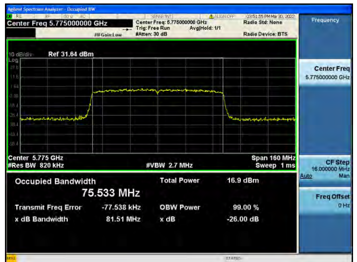
802.11ac_VHT80 UNII 3 BAND 26 dB Bandwidth (CH 155)
