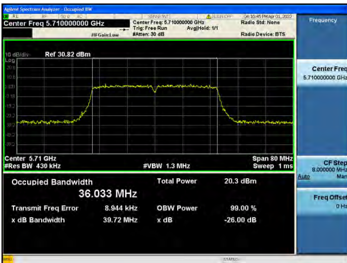
802.11ac_VHT40 UNII 2C BAND 26 dB Bandwidth(CH 142)
