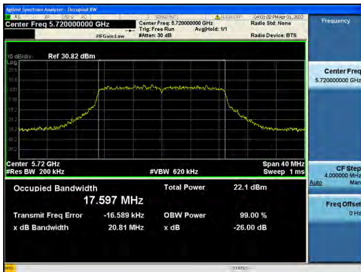
802.11n_HT20 UNII 2C BAND 26 dB Bandwidth(CH 144)
