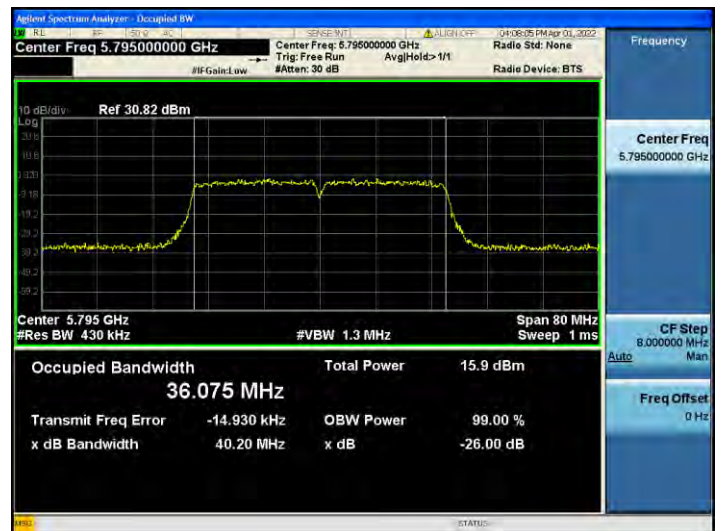
802.11n_HT40 UNII 3 BAND 26 dB Bandwidth (CH 159)
