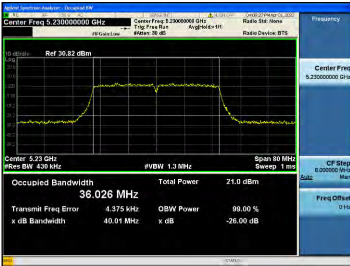
802.11ac_VHT40 UNII 2C BAND 26 dB Bandwidth(CH 142)
