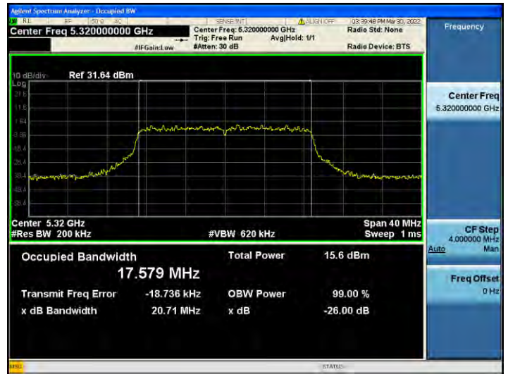
802.11n_HT20 UNII 3 BAND 26 dB Bandwidth(CH 149)
