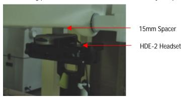
Note: the 15mm spacer was removed during the SAR measurement.
