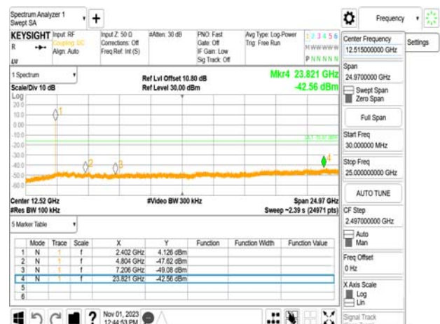
Spurious Emission_BLE 1M_LowCH00-2402MHz
