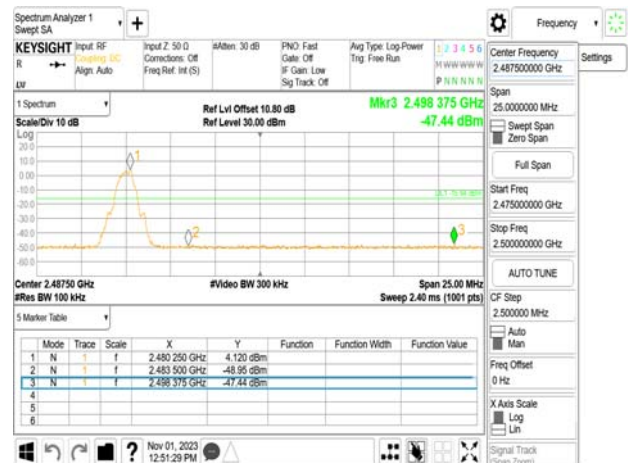
Spurious Emission_BLE 1M_LowCH00-2402MHz
