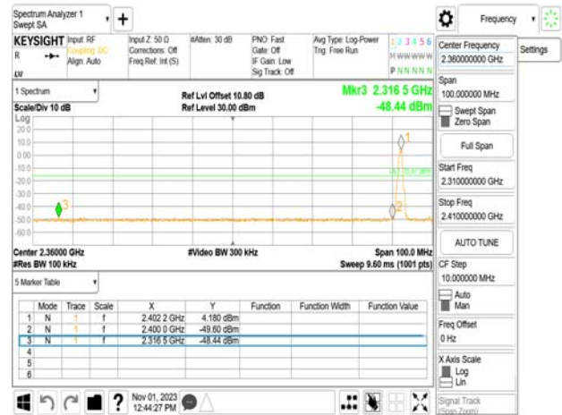
Band Edge_BLE 1M_HighCH39-2480MHz
