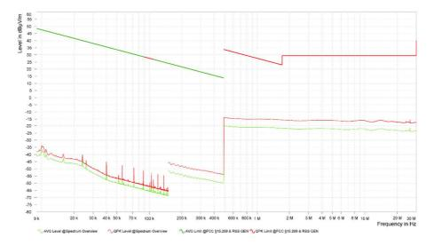
Remark: No emissions close than 20 dB to the limit, so no final measurement will be carried out.
