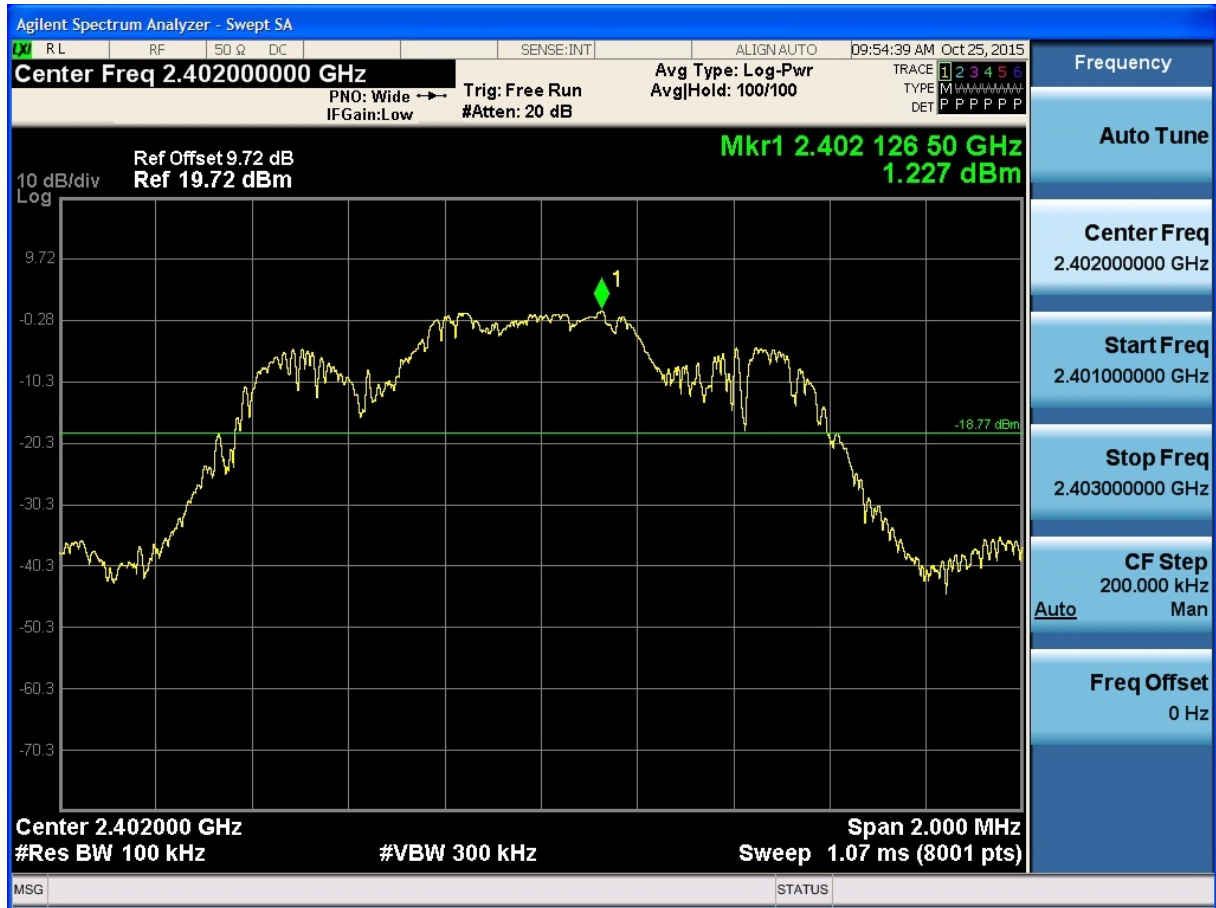
(Plot 4.9.2 A1: Channel 00: 2402MHz @ 8DPSK)
