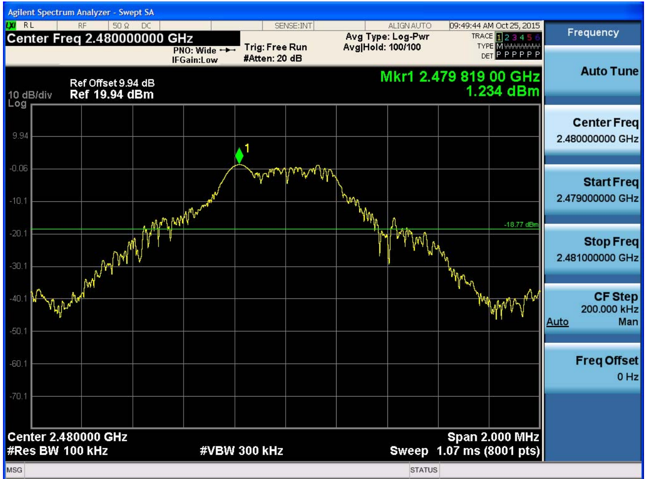
(Plot 4.9.1 C1: Channel 78: 2480MHz @ GFSK)
