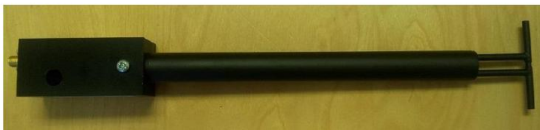
Figure 1 – MVG COMOSAR Validation Dipole
