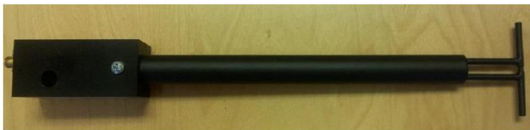
Figure 1 – MVG COMOSAR Validation Dipole
