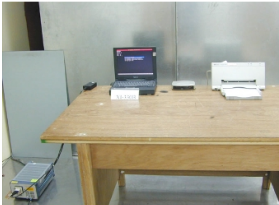
Photo 1: Conducted Test Set-up (front)
