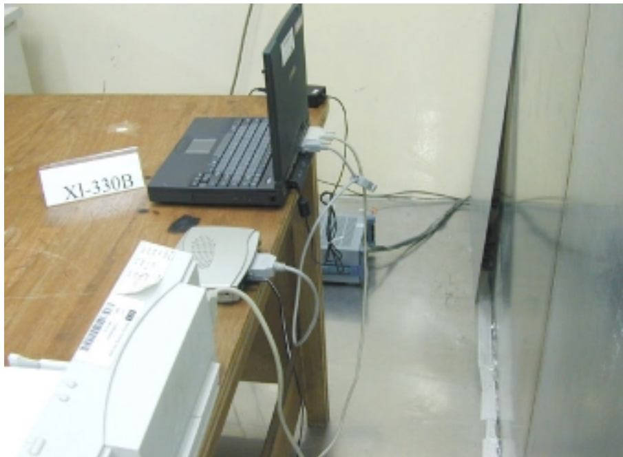
Photo 2: Conducted Test Set-up (rear)
