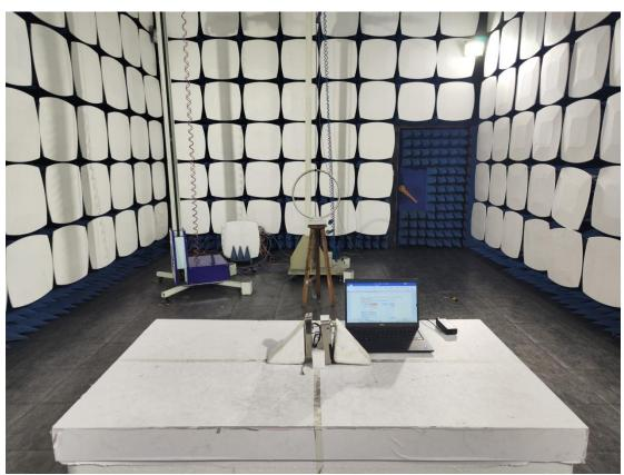
3. Radiated emission (9KHz-30MHz)
