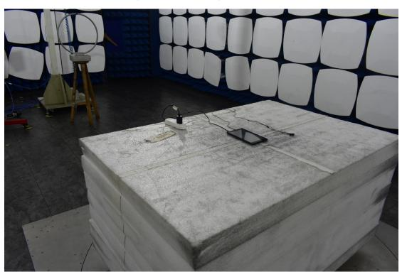
3. Radiated emission (9KHz-30MHz)
