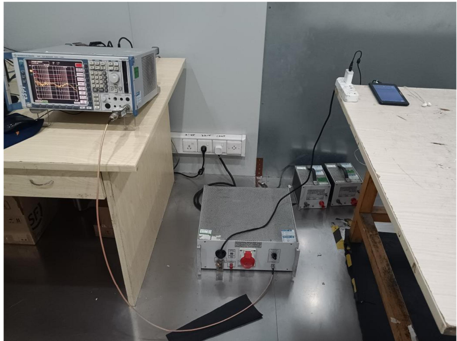
Conducted Emission Test Setup
