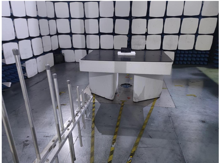
Radiation Emission Test Setup (30MHz to 1GHz)
