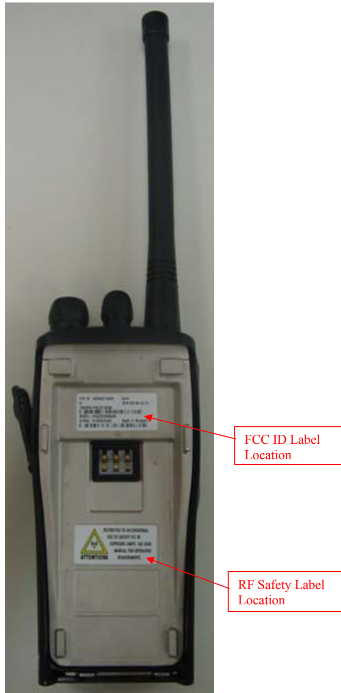
REAR VIEW WITH BATTERY REMOVED SHOWING FCC ID LABEL AND RF SAFETY LABEL
