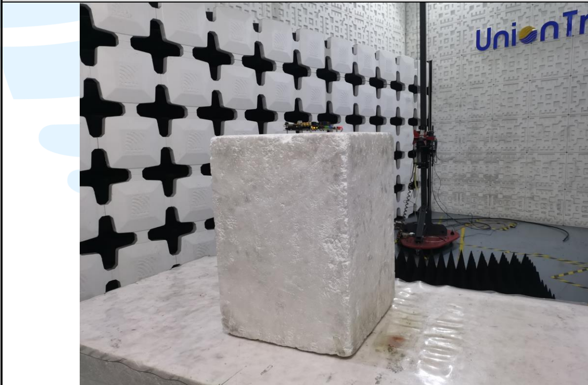
Radiated emission Test Setup(Above 1 GHz)
