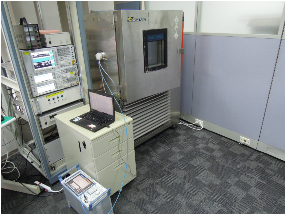
Photograph 6: Set-up for Conducted testing
