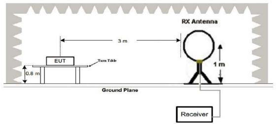
(2) Radiated Emission Test-Up Frequency 30MHz~1GHz
