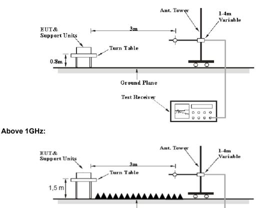
The radiated emission tests were performed in the 3 meters chamber test site, using the setup accordance with the ANSI C63.10-2013. The specification used was the FCC 15.209, and FCC 15.247 limits.
