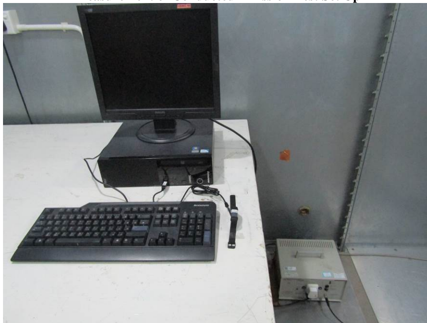
Measurement of Conducted Emission Test Set Up
