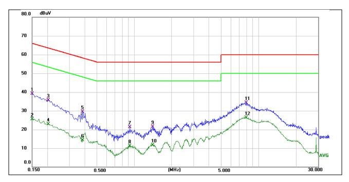
Phase: L1 Mode: BT 2M GFSK 2402MHz
