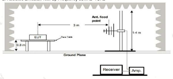
3. Radiated Emission Test-Up Frequency Above 1GHz
