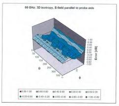
Probe isotropy for E<sub>tot</sub> probe rotated  $\varphi=0^\circ$  to 360°, tilted from field propagation direction  $\vec{k}$  Parallel to the field propagation ( $\psi=0^\circ$  - 90°) at 30 GHz: deviation within  $\pm$  0.38 dB Parallel to the field propagation ( $\psi=0^\circ$  - 90°) at 60 GHz: deviation within  $\pm$  0.33 dB
