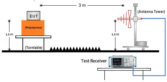
Above 1GHz Test Setup:
