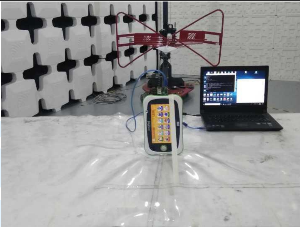
Radiated emission Test Setup (30 MHz~1 GHz)
