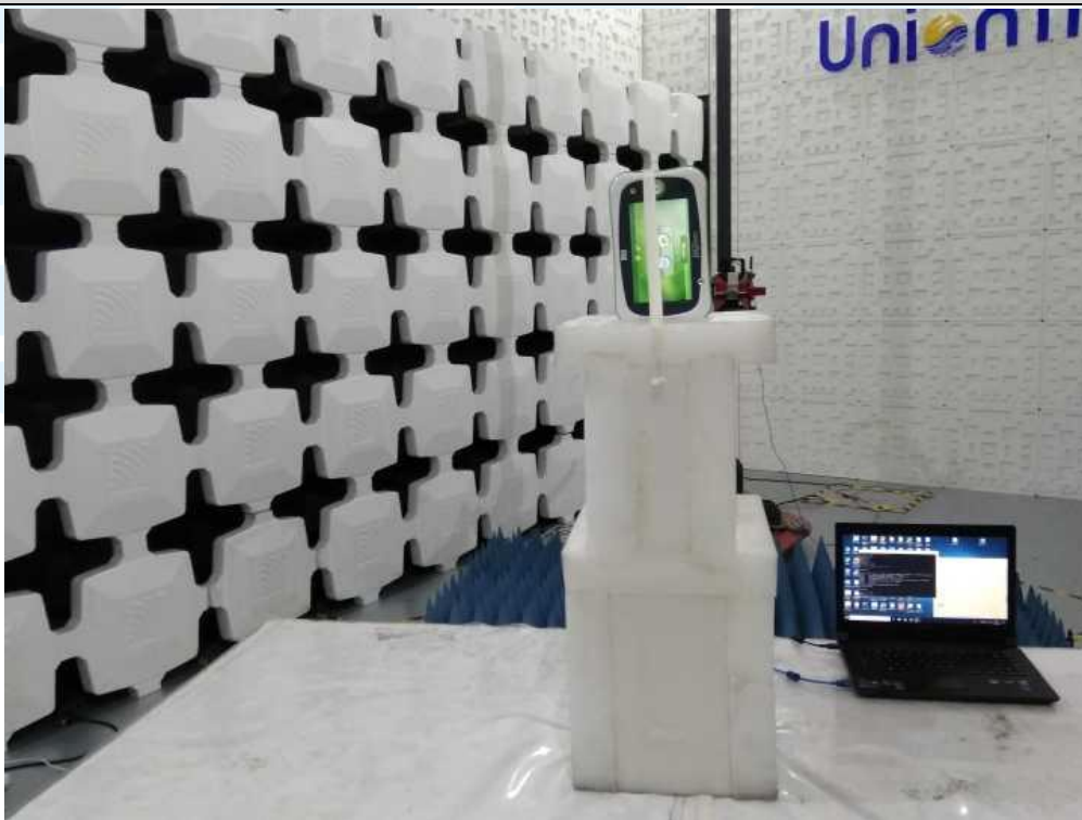
Radiated emission Test Setup (Above 1 GHz)
