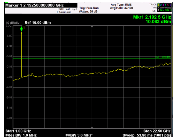
Channel: TOP, Modulation: QPSK, BW=15MHz, Range: Upper
