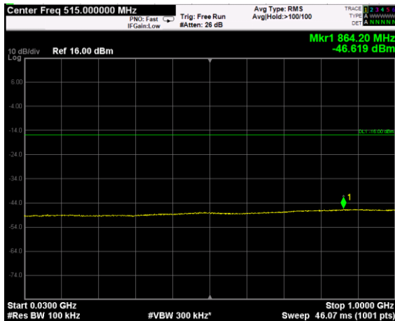
Channel: BOTTOM, Modulation: QPSK, BW=10MHz, Range: Lower
