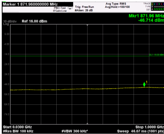
Channel: BOTTOM, Modulation: 64QAM, BW=15MHz, Range: Lower
