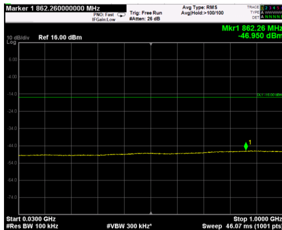
Channel: BOTTOM, Modulation: QPSK, BW=10MHz, Range: Lower
