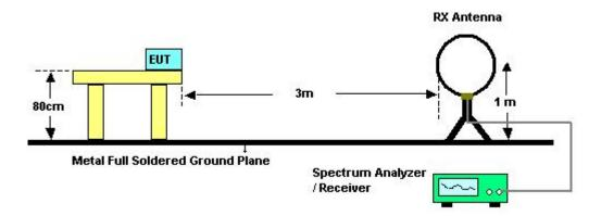
For Radiated Emissions: 30MHz~1GHz
