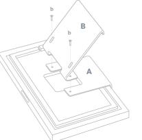
1. Attach the mount to the wall using the provided anchors and matching screws (c), with the pleat facing towards you.
