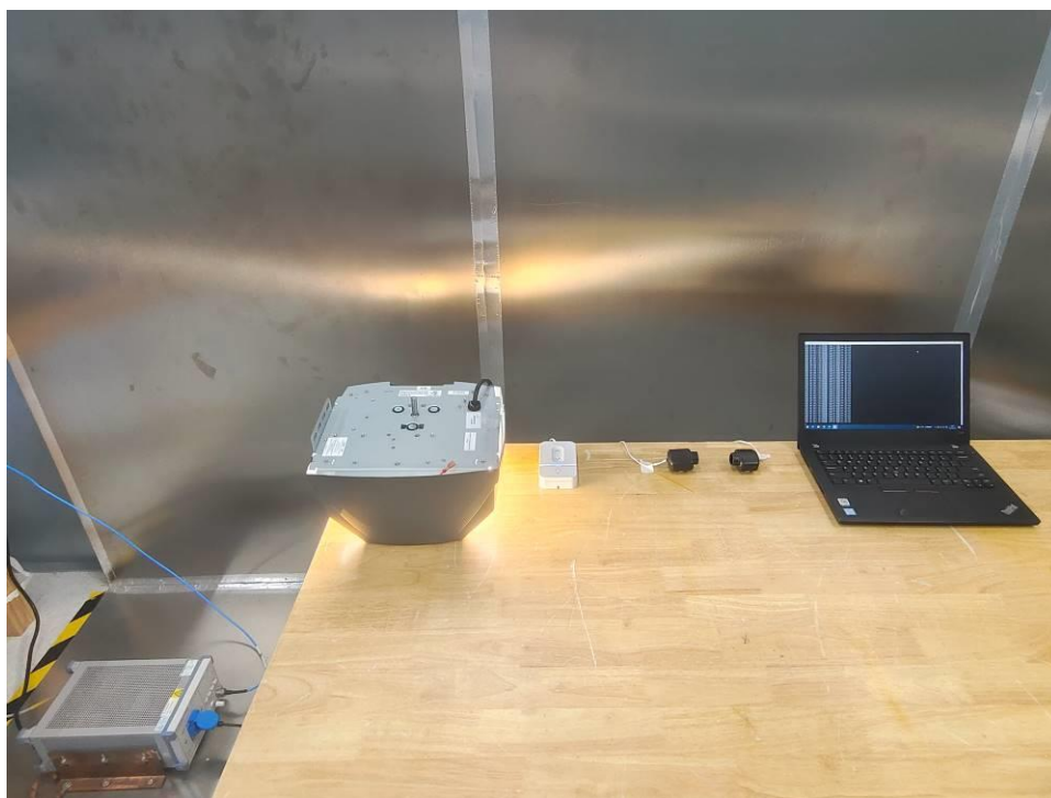
Photograph 1: Set-up for Conducted Emission on AC Mains
