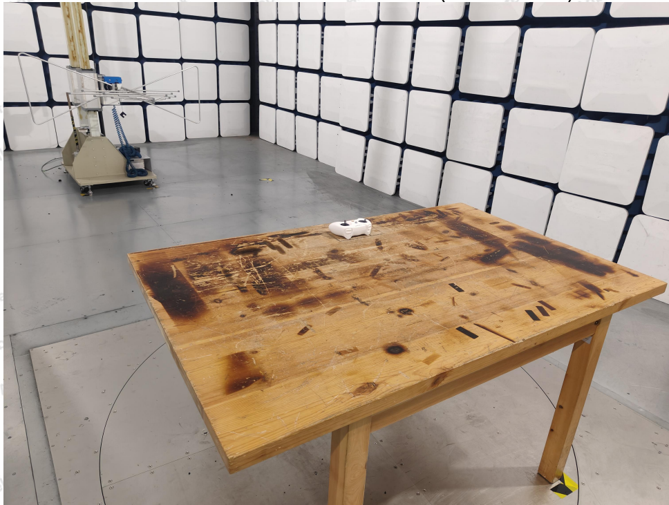
Photo of Radiation Emission Test (below 1GHz)
