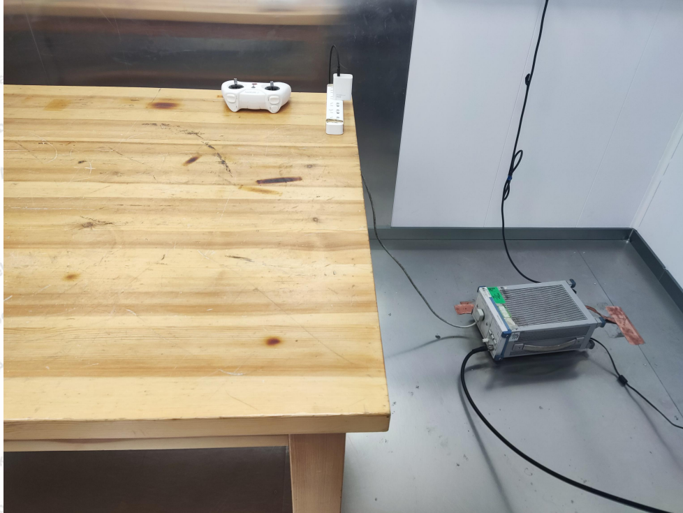
Photo of Radiation Emission Test (below 1GHz)
