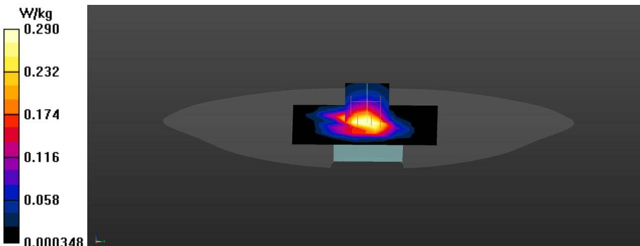
**LTE Band 4 20M QPSK 1RB-0 Back (0mm) Z-Axis plot**
