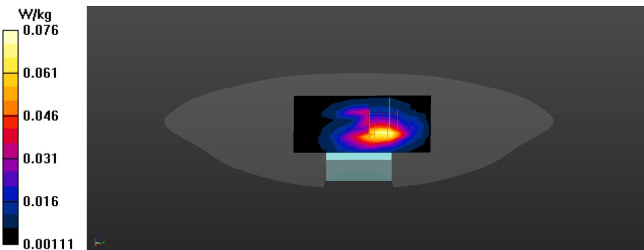
**LTE Band 12 10M QPSK 1RB-0 Front (10mm) Z-Axis plot****Channel: 23095**
