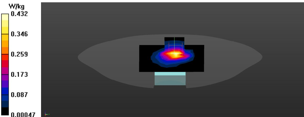
**LTE Band 4 20M QPSK 1RB-0 Front (10mm) Z-Axis plot**
