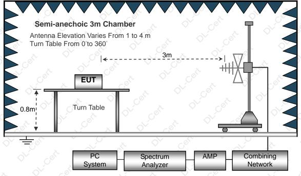
(C) Radiated Emission Test-Up Frequency Above 1GHz
