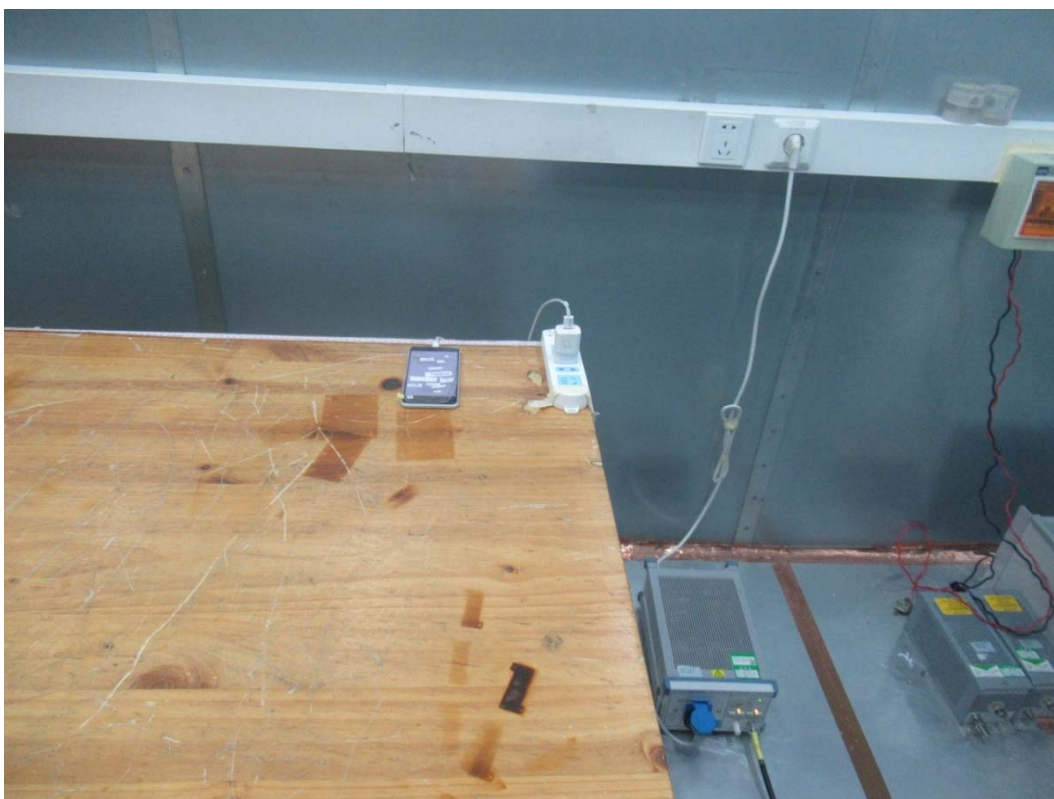
Picture 2 Conducted Emission Test Setup
