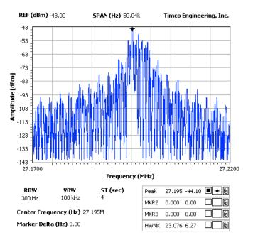
**METHOD OF MEASUREMENT:** A small sample of the transmitter output was fed into the spectrum analyzer and the attached plot was taken. The vertical scale is set to 10 dB per division.
