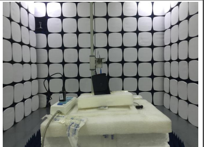
Radiated Spurious Emissions Test Setup Above 1GHz
