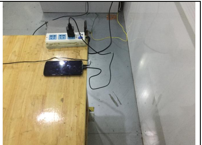
Conducted Emissions Test Setup Side View
