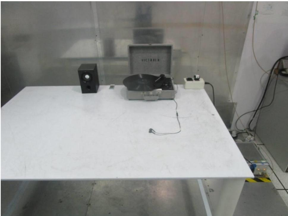
**Radiated Emissions & Radiated Emissions which fall in the restricted bands**
