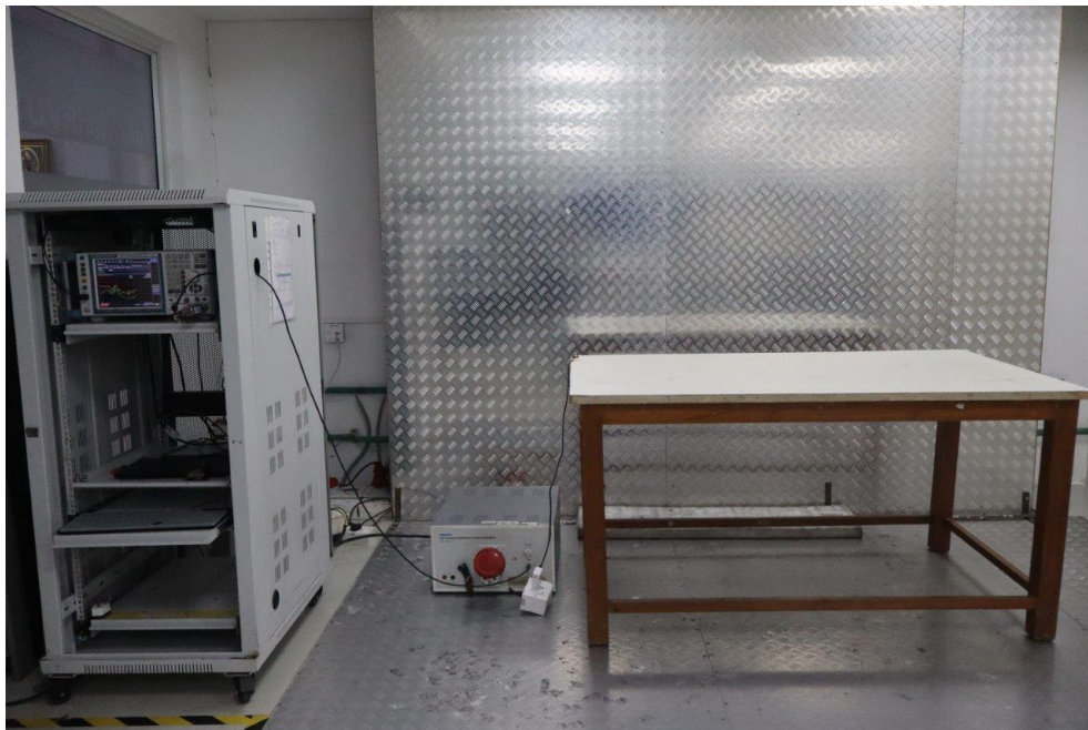
Conducted AC Power Line Test Setup
