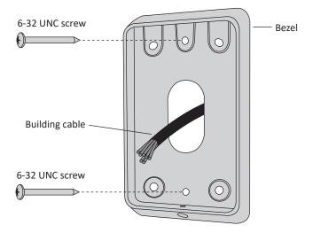
4. Connect the reader tail extending from the facia assembly to the building cable. Connect the wires for the appropriate reader you wish to interface, either an HBUS Reader or a Cardax IV Reader, as shown in the following diagrams.
