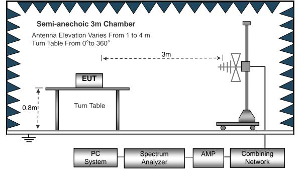
(C) Radiated Emission Test-Up Frequency Above 1GHz
