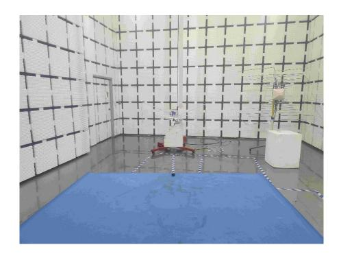
Conducted Emissions at AC Power Line (150kHz-30MHz)
