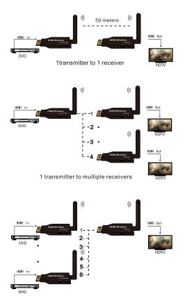
Multiple transmitters to one receiver support a maximum of 6 to 1.
