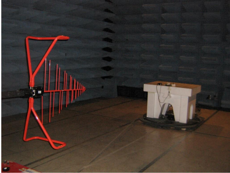
Radiated Emissions Test Setup - 30MHz-1GHz
