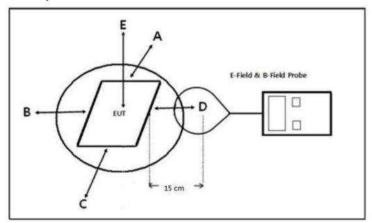
Note: Position A: Front of EUT; Position B: Left of EUT; Position C: back of EUT; Position D: Right of EUT; Position E: Top of EUT(20 cm measure distance);
