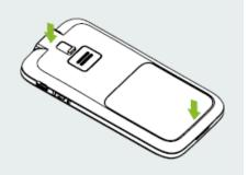
• First time start up: Press and hold the power button, the PDA will vibrate, indicating that the PDA is powered on. After about 30 seconds the Setup Wizard will appear and guide you through entering basic settings.
