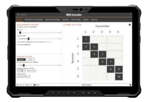
The computer or tablet used for measurements should be placed in a convenient position for the operator to monitor the measurement progress whilst carrying out the investigation. An Ethernet cable is used to transfer the measured data from the system to the data acquisition computer or tablet for storage and display in MIRA Controller.
