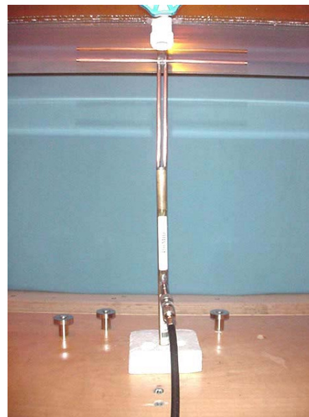
450 MHz Dipole Setup
