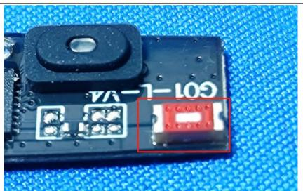
The antenna is Ceramic antenna.
