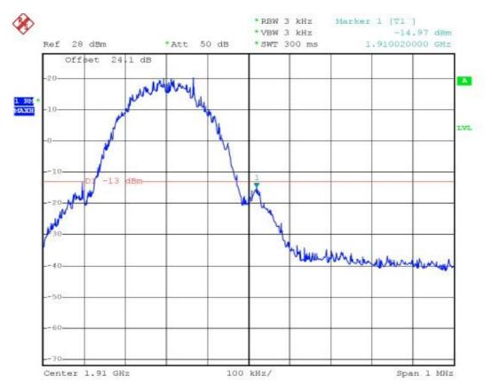
**Name of Test**: Emission Masks (Occupied Bandwidth) State 2:High Power
