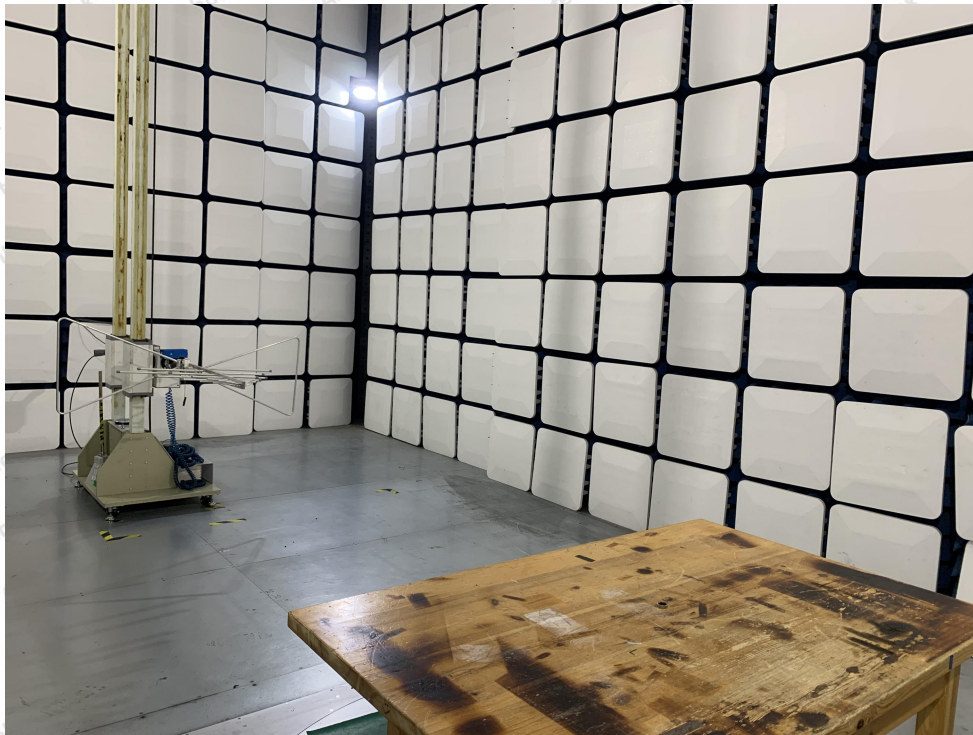
Photo of Radiation Emission Test
