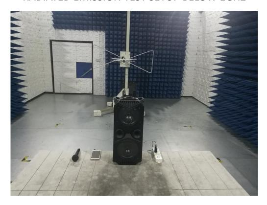
RADIATED EMISSION TEST SETUP ABOVE 1GHZ
